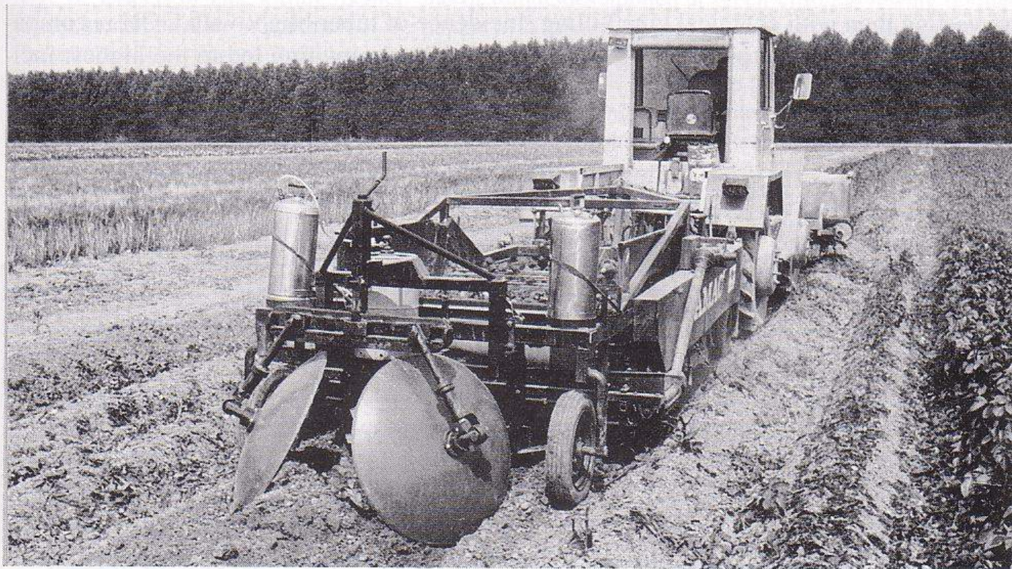
Fig. 2. Green-crop-harvesting in operation. The two containers on the rear serve to treat the collected tubers with antagonists and/or fungicides.
